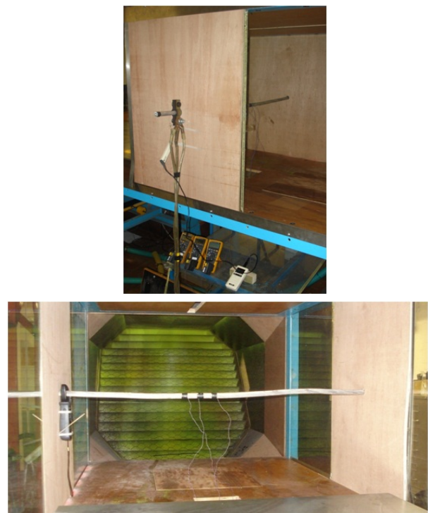
Fig. 3 External and internal view of wind tunnel test rig
